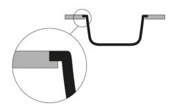
**Drop-On Sink Fitment** sinks are designed to be easily fitted to any type of worktop material. They have self-rimming flanges which will conceal the core layer of a laminated worktop.
